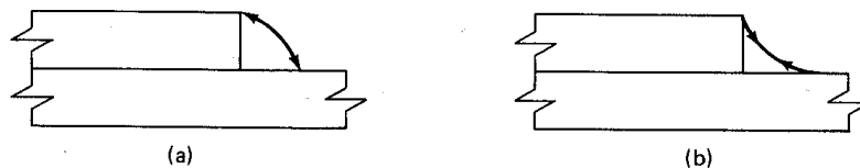
Figure 8.14 Fillet welds with convex and concave surface. (a) Convex surface under compression; (b) concave surface under tension
