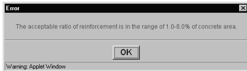
Figure 4.12 Applet warns the user when the entered reinforcement ratio is not a practical one
